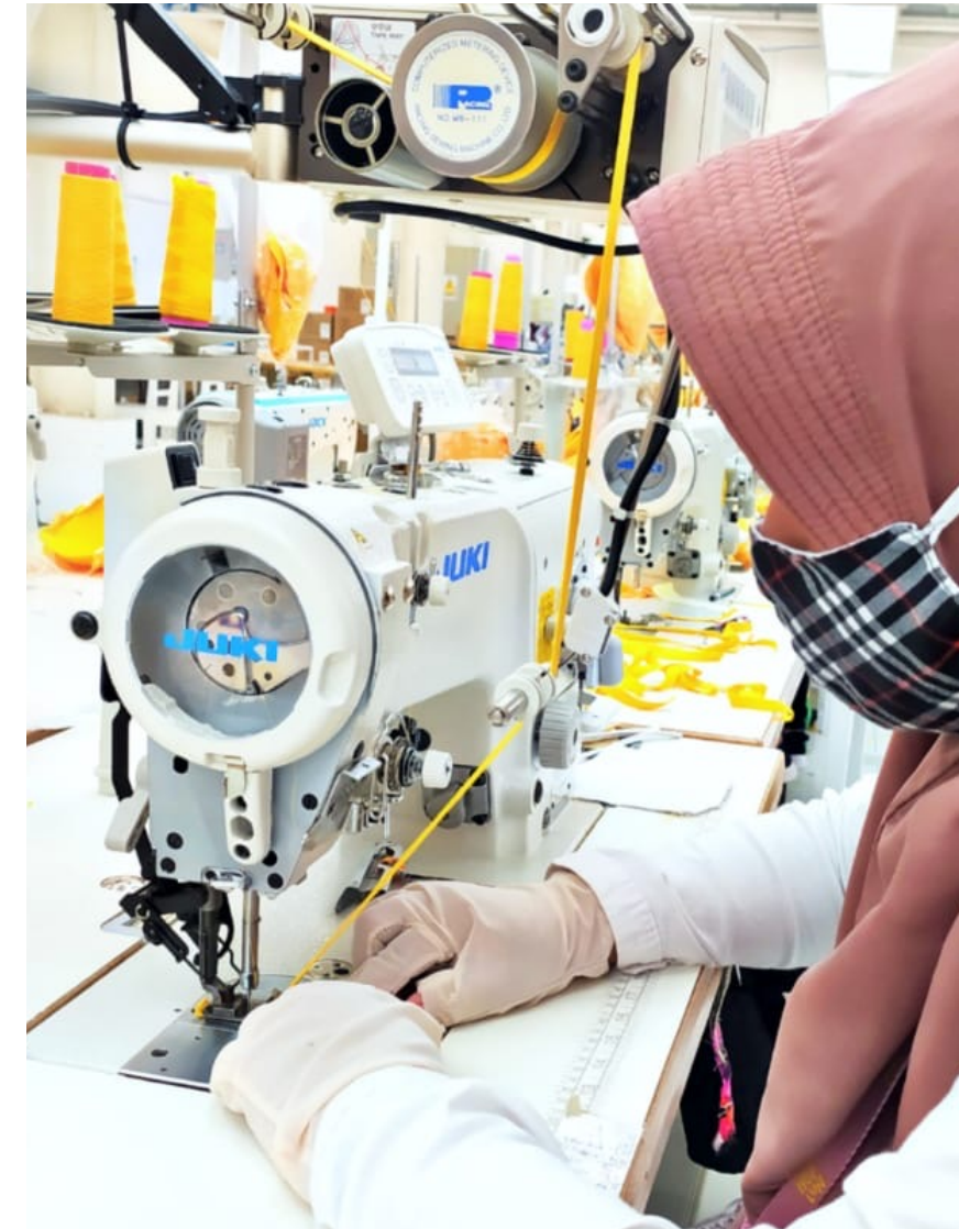
A new sewing machine with a built-in servomotor saves 30% energy compared to a conventional sewing machine.
